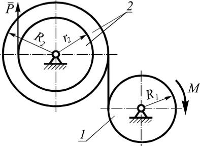
25. Find the angular acceleration of the body 2, if  $m_1, m_2, R_1, R_2, r_2, i_{1x}, i_{2x}, P$  and  $M$  are known.
