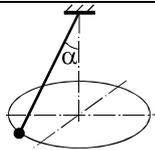
29. The motion trajectory of a material point of mass  $m$  in the horizontal plane is equal to a circle. The point is hanged by a thread of length  $l$ , the angle of deviation from the vertical is  $\alpha$ . Find the velocity of the point.
