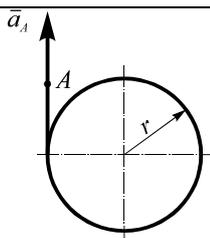
30. The thread is wound on the homogeneous cylinder of mass  $m$  and radius  $r$ . A free end  $A$  of the thread moves vertically with a constant acceleration  $a_A$ .
