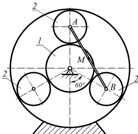
For the shown position of the planetary mechanism the angular velocity and angular acceleration of the central wheel 1 are  $\omega_1$  and  $\varepsilon_1$  respectively. The radius of wheel 1 is  $r_1$  and the radius of wheel 2 is  $r_2$ .
