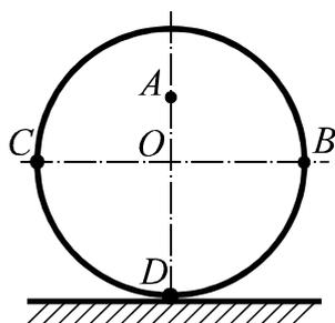
Disk of radius  $r$  is rolling on a horizontal surface with slipping. It has a constant angular velocity. The points  $A$  and  $B$  have the same velocity and acceleration.  $OA = r/2$ .
