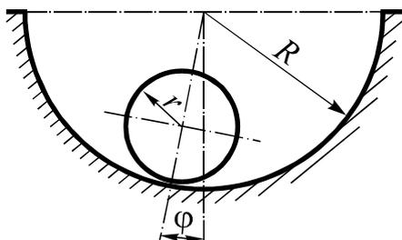
A solid homogeneous disk of radius  $r$  rolls without slipping along the arc of a circle of radius  $R$ . Find out the velocity which should be given to the center of the disk at its lower position for the decreasing of the normal cylinder pressure force in 1.5 times for the position of the disk when the angle  $\varphi = 60^\circ$ .
