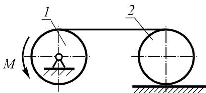
Homogeneous cylinder 1 rotates around a fixed axis under the action of pair of forces. It is connected with the same cylinder 2 with a non-stretchable thread. The cylinder 2 rolls on a horizontal surface.
