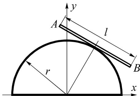
Homogeneous thin rod  $AB$  of length  $l$  is based on the half-cylinder of radius  $r$ . Static friction coefficient between the rod and the half cylinder is equal to  $f$ , the coefficient of rolling friction is  $\delta$ .
