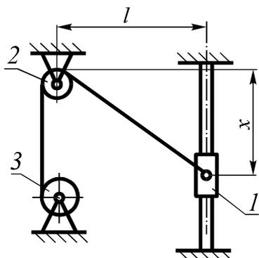
The load 1 of mass  $m$  rises along the vertical rod by the rope thrown over the block 2 (its sizes can be neglected). The block 2 is hanged at a distance  $l$  from the rod. The coefficient of friction between the load 1 and the rod is  $f$ . Determine the dependence of the rope tension force  $T$  on the distance  $x$ , if the rope is wound on a uniformly rotating wheel 3 with a linear velocity  $v_0$ .
