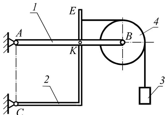
The construction shown in the figure consists of two weightless rods 1 and 2, which are connected at point  $K$  by a hinge. The load 3 is linked with the rod 2 by the weightless thread thrown over the block 4. The load 3 and block 4 have the same mass. Block 4 has the radius  $r$ ,  $KB = 2r$ ,  $AK = 3r$ .
