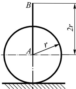
The homogeneous disk with radius  $r$  is fastened with thin homogeneous rod  $AB$ . The disk and rod have the same masses. In the depicted position the quiescent system begins to move under the gravity forces. Ignoring the friction between disk and surface define the velocity of rod end  $B$  at the moment of the impact against the surface.
