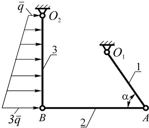
In the bar system placed in the vertical plane the homogeneous rods 1, 2 and 3 have lengths  $l_1$ ,  $l_2$ ,  $l_3$  and gravity forces  $G_1$ ,  $G_2$ ,  $G_3$  respectively. In equilibrium position rod  $AB$  is horizontal, rod  $O_2B$  is vertical and the angle between rods  $O_1A$  and  $AB$  is  $\alpha$ . Define the value  $q$  for the intensity of the distributed load with linear variation when the given equilibrium position of system is provided.
