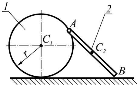
Disk 1 with radius  $r$  is rolling along the horizontal surface without slipping so that the speed of its centre  $C_1$  is constant. Rod 2 with length  $2r$  is hinged to point  $A$  of the disk rim, rod end  $B$  is sliding along the surface. Define how many times the speed of  $C_2$  rod centre is higher than the speed of  $C_1$  disk centre at the moment when point  $A$  is at its highest position.
