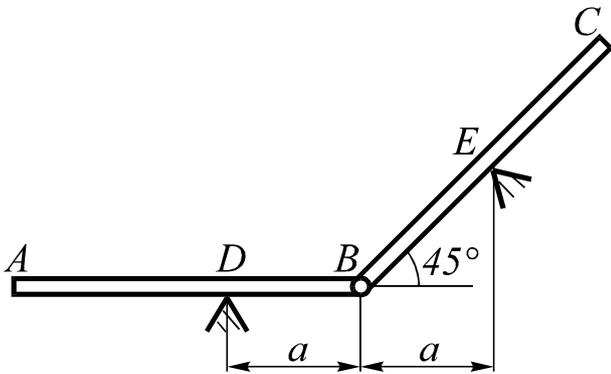
Two homogeneous rods  $AB$  and  $BC$  with the same masses are connected by hinge at point  $B$  and placed on two rough edges  $D$  and  $E$ . Define the rod lengths when the equilibrium in the depicted position is possible if the coefficient of friction between the rods and supports is  $f$ , and size  $a$  is also known.
