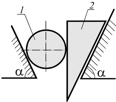
Cylinder 1 with mass  $m_1$  and wedge 2 with mass  $m_2$  touching each other are moving between two inclined surfaces forming the identical angles  $\alpha$  with the horizon. The frictions between the cylinder and the wedge as well as between the wedge and the surface are negligibly small. The cylinder is rolling along the inclined surface without slipping. Define what force the cylinder applies on the wedge.
