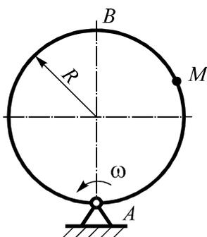
Disk with radius  $R$  is rotating about the motionless axis with the constant angular velocity  $\omega$ . Along the disk rim particle  $M$  is moving from  $A$  to  $B$  with constant relative velocity  $v_r = \sqrt{3}\omega R$ . Define the radius of path curvature for the absolute motion of particle  $M$  in the position when the relative and transport velocities are the same.
