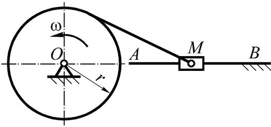
The pulley with radius  $r$  is rotating about its axis with the constant angular velocity  $\omega$ . The pulley is wound with the thread to the free end of which slider  $M$  is attached. The slider with mass  $m$  is moving along rod  $AB$  the extension of which crosses the pulley axis at right angle at point  $O$ . The coefficient of friction between the slider and the rod is  $f$ . Define the thread tension force with distance  $OM = x$ .
