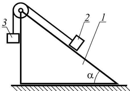
Prism 1 with mass  $m_1$  may slide along the smooth horizontal surface. Two loads 2 and 3 with masses  $m_2$  and  $m_3$  ( $m_2 \sin \alpha > m_3$ ) are connected by inextensible thread and sliding along the inclined and vertical prism faces respectively and the friction between load 2 and the prism is negligibly small. The coefficient of friction between load 3 and the prism face is  $f$ . Define the acceleration for prism 1. Block weight can be ignored. Angle  $\alpha$  is known.
