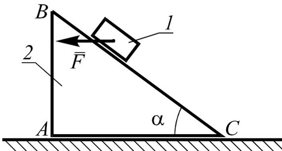
The load 1 with the mass  $m_1$  is sliding along the face of the prism 2 with the mass  $m_2$  moving along the horizontal plane. The friction between the bodies is absent. The angle  $\alpha$  is known. Find the minimal horizontal force  $F$  when the prism turn-over begins (i. e. the point C breaking-off from the surface).
