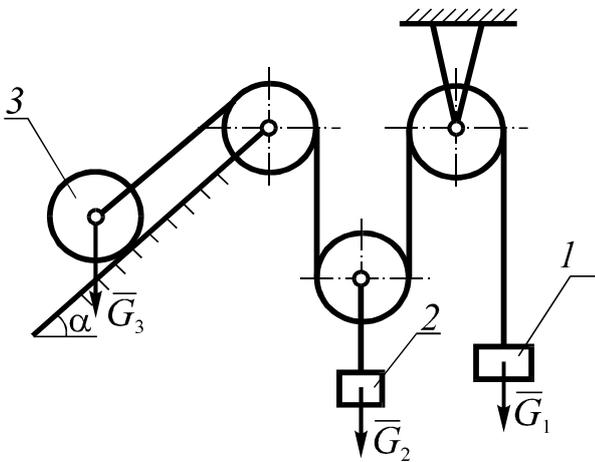
What is the weight of load  $G_1$  in order that the load 1 is motionless in the mechanical system when  $G_2 = 3G$ ,  $G_3 = G$ . Ignore the masses of unnumbered blocks, cables and friction in hinges. Consider the body 3 as a solid homogeneous disk. The coefficient of friction between the disk 3 and the surface is  $f$ . The angle  $\alpha$  is given.
