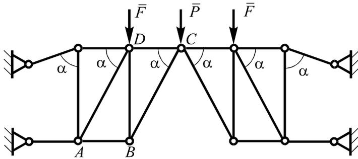
In the depicted rod construction all rods are weightless. Find at what proportion of the internal forces  $F$  and  $P$  in the rods  $AB$  and  $CD$  are 5 times different.  $\alpha = 60^\circ$ .
