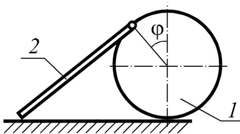
The homogeneous disc with the mass  $m_1$  and the radius  $R$  is hinged to the homogeneous rod with the mass  $m_2$  and the length  $l$ . Define the minimal constant of friction between the bodies and the surface when the system is in equilibrium in the position defined by the angle  $\varphi$ .
