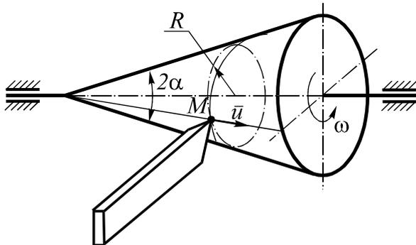
The lathe tool is doing translational displacement along the cone with the constant velocity  $\bar{u}$ . Define the radius of motion path curvature for the tool point  $M$  in regard to the cone in the place where its radius is  $R$ . The cone is uniformly rotating with the angular velocity  $\omega$  on the fixed axis and the vertex cone angle is  $2\alpha$ .
