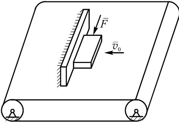
The load with the mass  $m$  on the conveyor belt is moving crosswise under the constant force  $F$ . The immovable barrier interferes with the lengthway movement of the load. The coefficient of friction between the load and the belt is  $f_1$ , between the load and the barrier is  $f_2$ . The speed of the belt is  $v_0$ .
