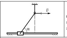
11. The rope put through the hoop is fastened to the slider which can be moving along the guideway. The rope is with the velocity v. Define the slider velocity at the moment when the rope makes the angle  $\alpha$  with the horizontal.
