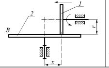
15. In a friction mechanism shaft 1 with radius *r* is revolving with uniform angular acceleration  $\varepsilon_1$  and at the same time is moving in the line indicated by the arrow. According to which law of distance variation *x* disk 2 will be revolving with uniform angular velocity  $\omega_2$  if at the initial time  $x_0 = a$ ?
